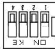
Figure 3-7 Boot-up from SPI Flash
