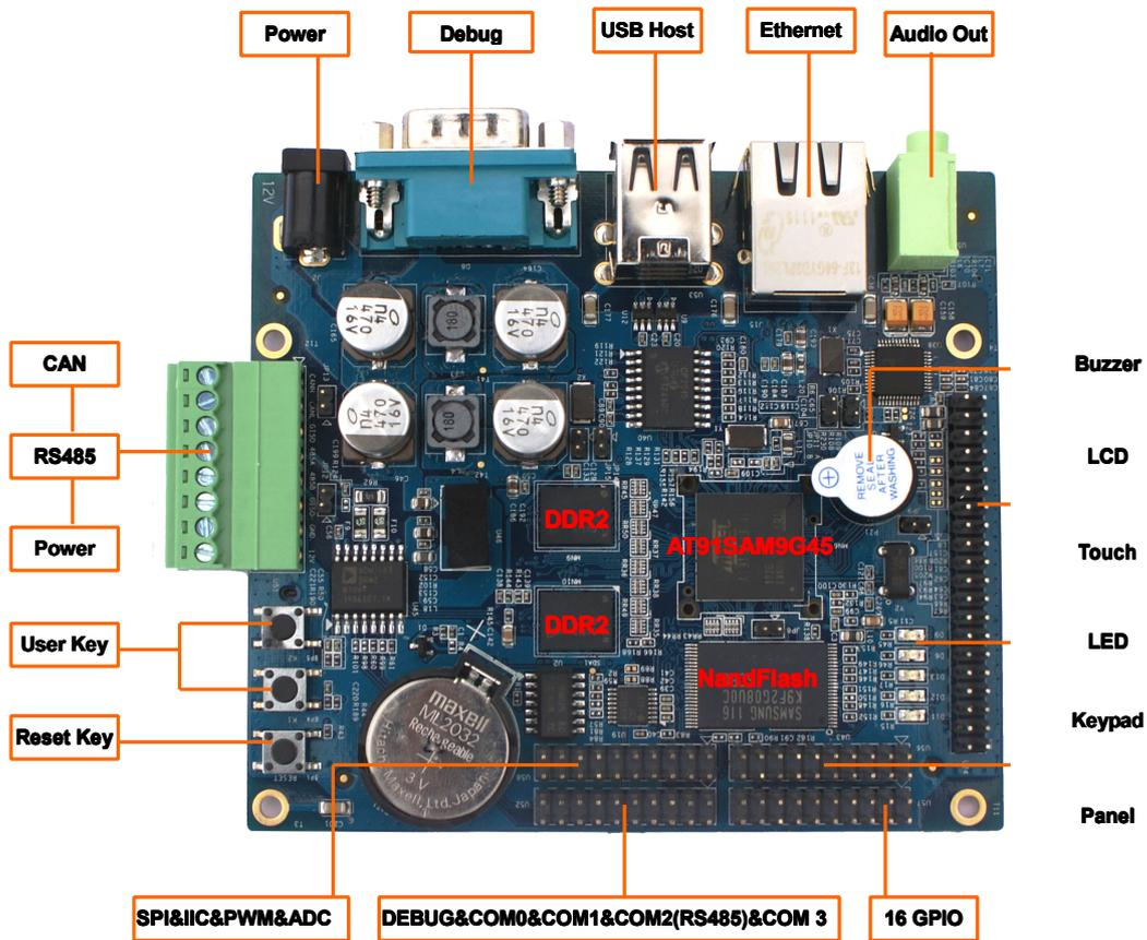
**Figure 1-1** Components on SBC6845
