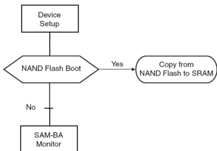
**Figure 2-1** System Booting Process
