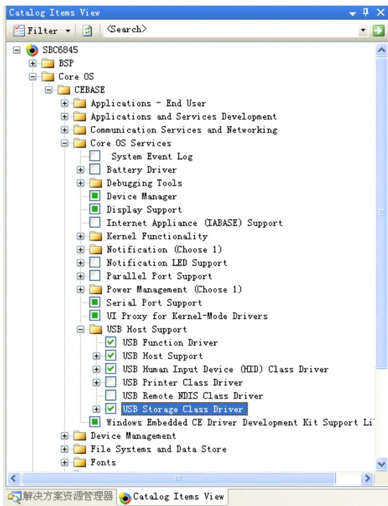
**Figure 2-11** Customization Configurations
