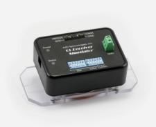
The Qi FOD Receiver is a low power receiver that can be used to test the operation and FOD performance of Qi wireless transmitters. DIP switches on top of the FOD Receiver are used to program received power offsets and to change internal loads.
