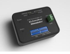
The Qi Receiver Simulator is a low power receiver that can be used to test the operation and performance of Qi wireless power transmitters. DIP switches on top of the Qi Receiver Simulator can be used to select different operational test modes as well as select different communication modulators and internal loads.
